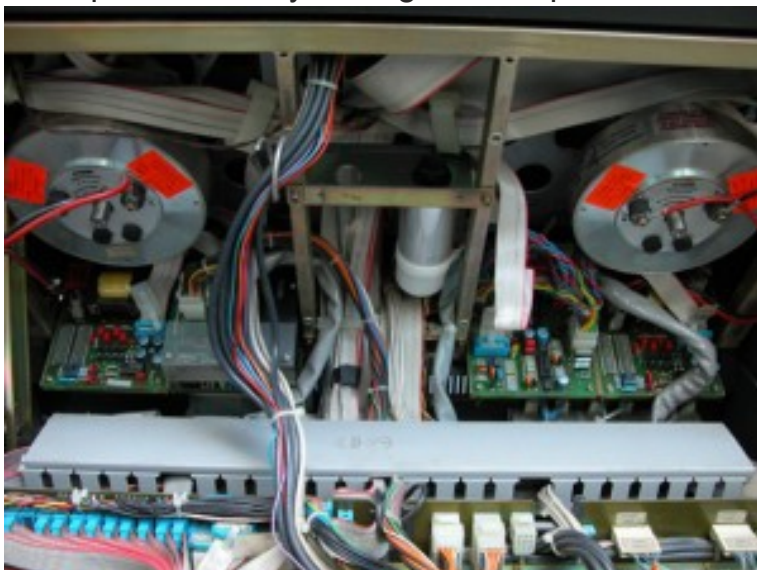
From a Studer A820: The underside of the reel motors, with an MDA motor driver and electronics below.
