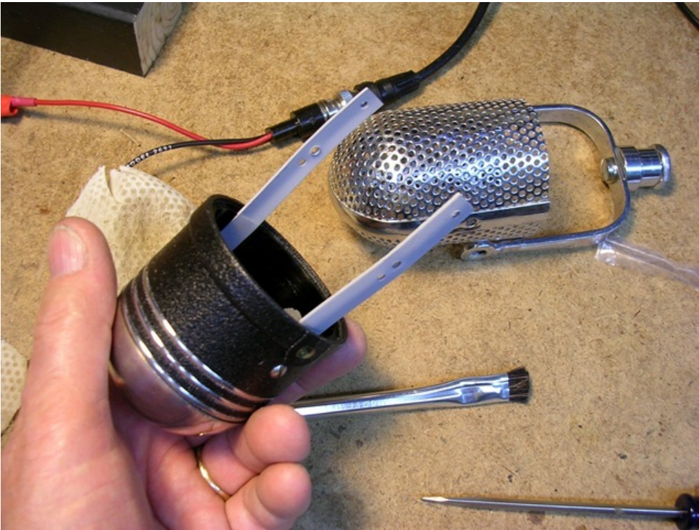
4. This is the mic case, puttied and repainted.
