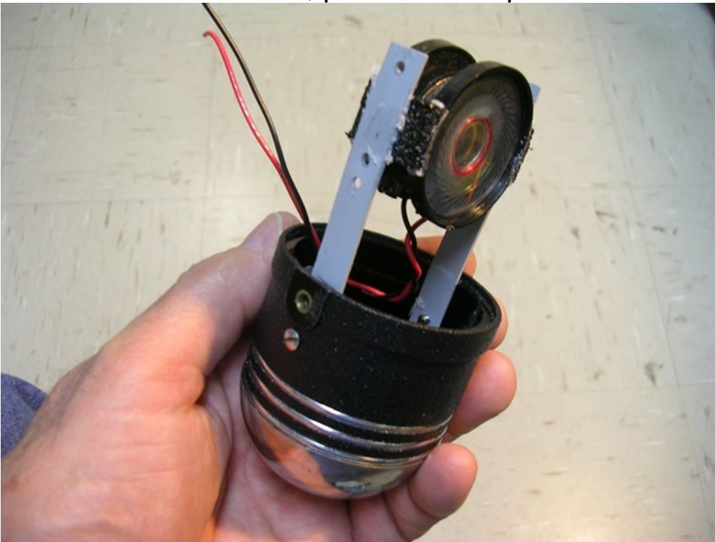
5. And how the dynamic elements were mounted and wired in proper phase to give a ribbon-like bidirectional pickup pattern.
